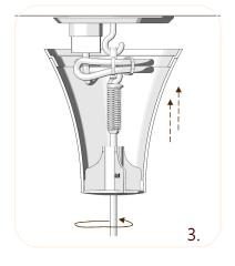
Screw the lamptop onto the screw. It is then directed straight upwards and with the ceiling hook as anchorage, it sits perfectly.
