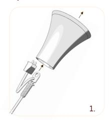
Fasten the cord into the semi-open screw, enter through the lamptop and hang on the ceiling hook.
